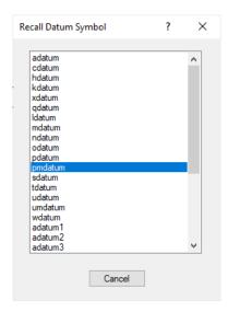
This pmdatum can be placed on a part or on a nest. The location of the pmdatum will be used as the 'bottom left' corner of the mark.
