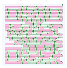
The sequence is fixed and can use fly-cutting if the machine / postprocessor supports it.
