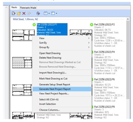
From the nest panel, a new option allows the user to quickly issue a new version of the nest project report as a PDF file. The folder location is specified in the machine settings:
