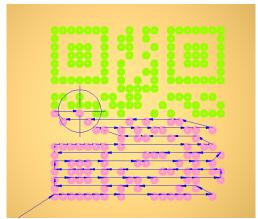
On profiling machines, the GPP can automatically output fly-cut codes for part marks even if the user doesn't use 'FLYCUT SCAN' in the order text. We have found that the use of fly-cutting is recommended on MAZAK machines.
