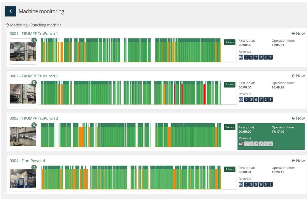
Here it is instantly visible if machine is operating (green), being setup (yellow), setup time has been exceeded (flashing orange) or production has been interrupted (flashing red).
