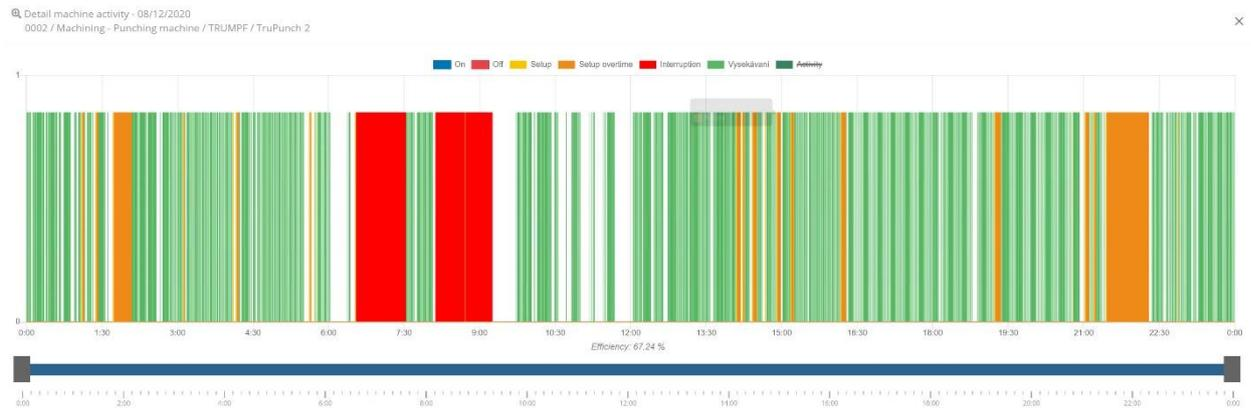
ZOOMFAB allows operator or supervisor to record the cause of interruption with two clicks. First one is to identify the interruption on zoomed graph, the second one to identify cause (it is also possible to identify multiple causes in one go).
