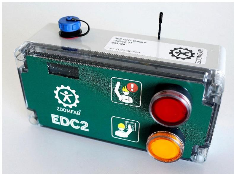
EDC2 requires independent electricity connection (220VAC or 24VDC) located close to the machine. This will allow unit to operate even when machine is switched OFF. There is no other connection required, as unit communicates wirelessly with standard ZOOMFAB gateway.
